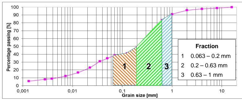
Fig. 3 Grain size distribution curve and used fractions
