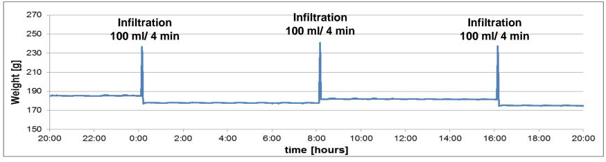
Fig. 6 Changing of water content due to 3 infiltrations over 24 hours in the soil with grain size fraction 0.63 - 1 mm
