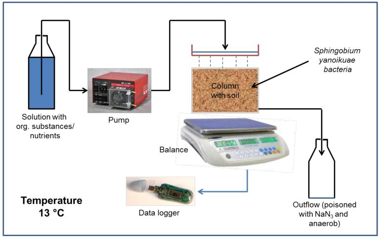
Fig. 2 Experimental setup
