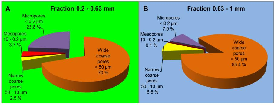
Fig. 5 Distribution of pores sizes in grain size fraction 0.2 - 0.63 mm (A) and 0.63 - 1 mm (B)
