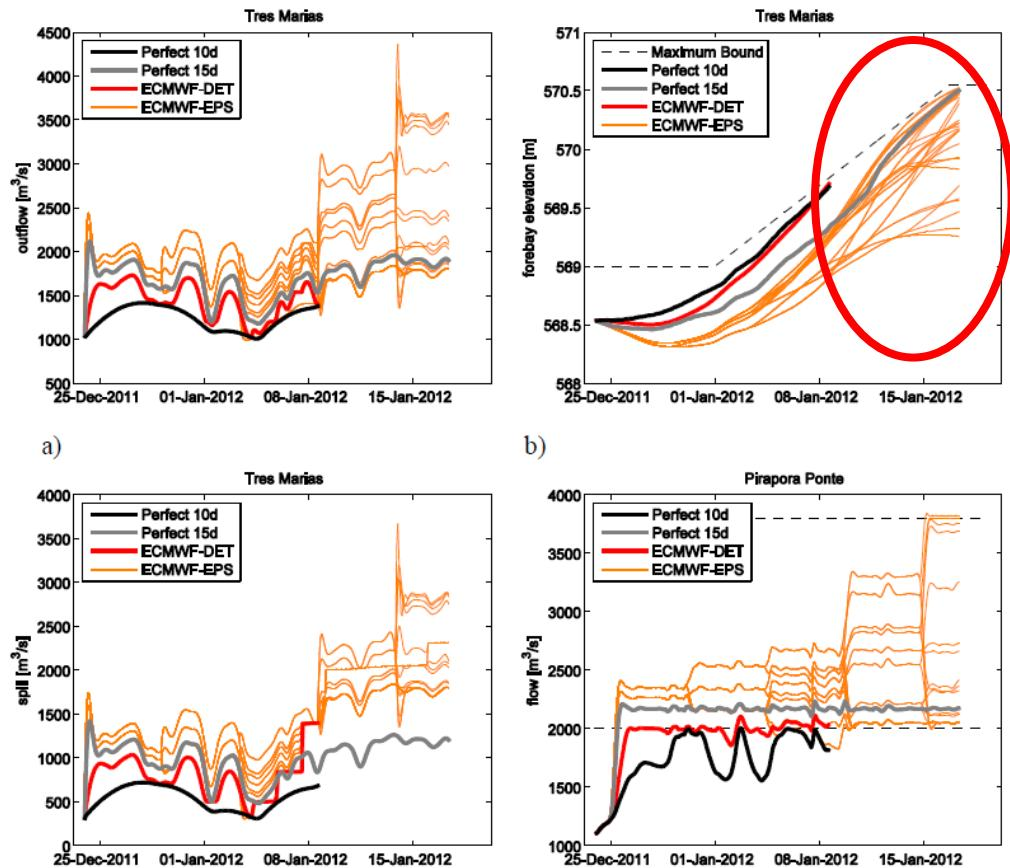
Stochastic optimization showed a more conservative allocation of storage due to the forebay elevation hard constraint. The control trajectory of the stochastic optimization meets the constraint for all 32 branches of the scenario tree.
