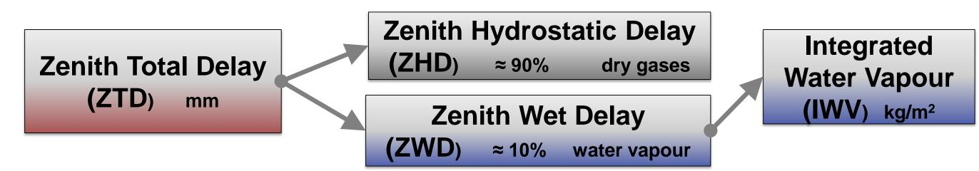
ZTD is determined from the sum of the two components, ZHD and ZWD. Usually ZHD varies very slowly in time and can be very accurately estimated using surface pressure measurements at the GPS station. ZWD is highly variable given the variability of the water vapour and the deficiencies in its observations. For this work we use the GAMIT\GLOBK software (v10.5) to process the GPS data in daily solutions.
