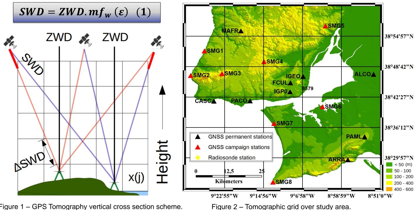
Figure 1 – GPS Tomography vertical cross section scheme
