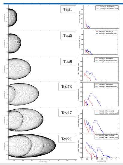
The length of the deposit is even longer from flow to flow. It is link to the increasing velocity in the channel.
