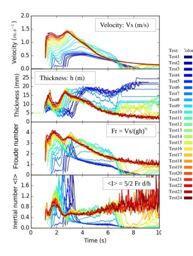
The maximum velocity increases for all the tests. For the first tests (1-5) there is only one front velocity measure then for the other tests two front are detected with two peaks.
