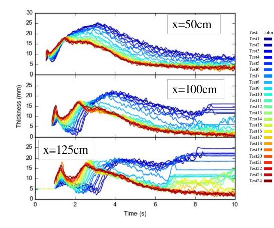
Sensor 1 (x=50cm) show an analogous behavior for the head flow. But for the first tests (1-5) the tail front form a deposit in the channel while for the latter (18-24) there is no more beads.
