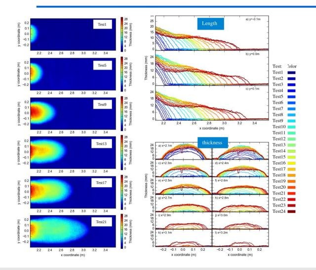
Length: The measured thicknesses of the deposit clearly show the increase of the run-out distance from test to test.
