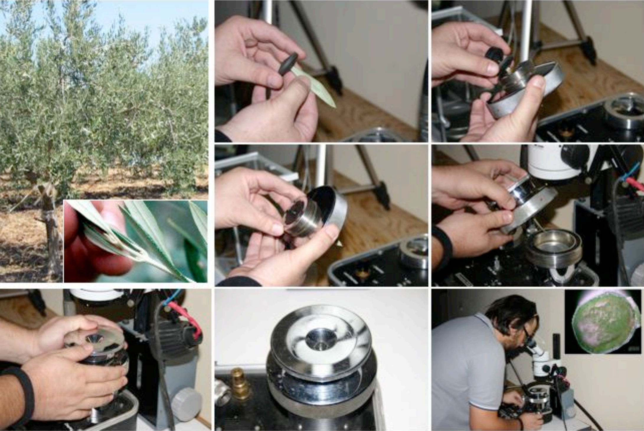
Fig. 3 – Measurements of Leaf water potential
