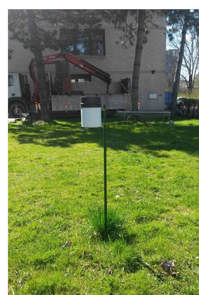
Tipping bucket rain gauge
