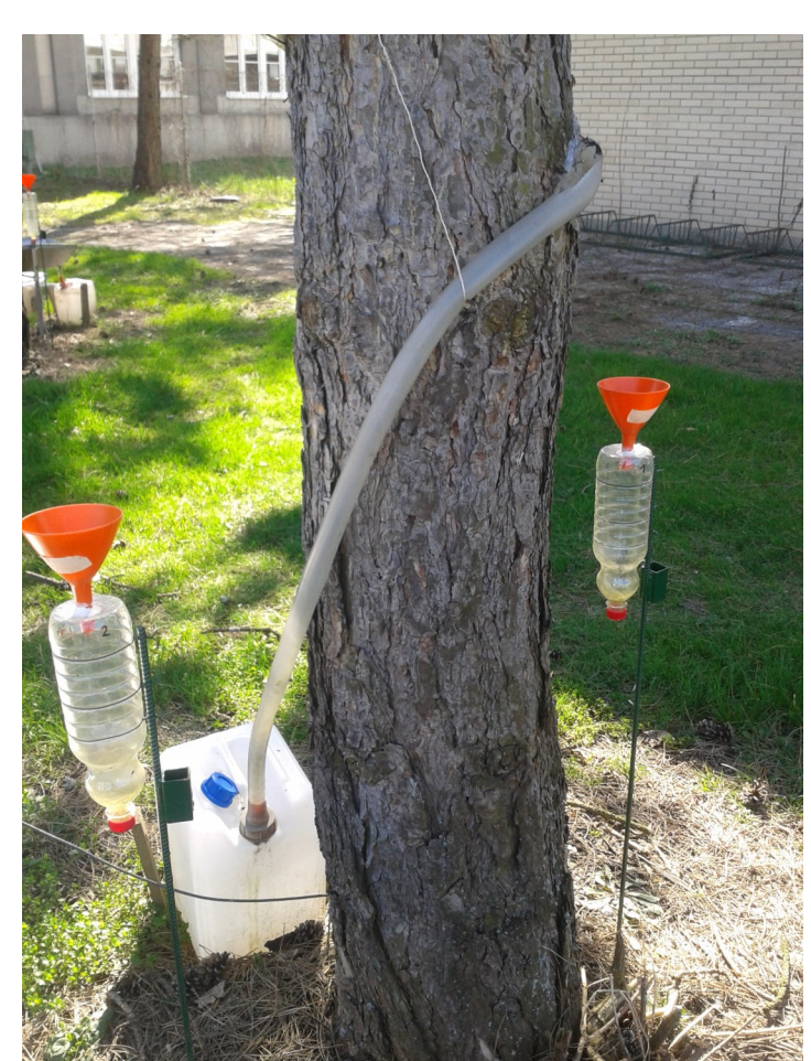
Measurement of stemflow and manual roving gauges
