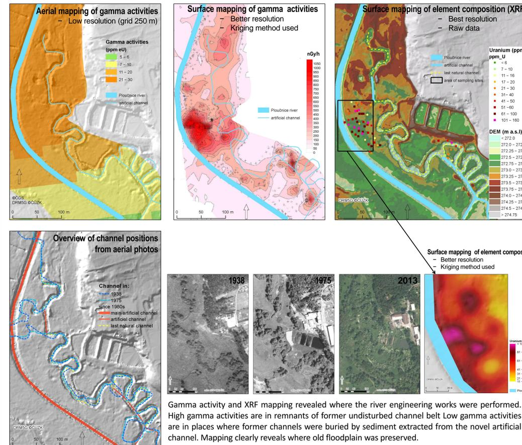
Gamma activity and XRF mapping revealed where the river engineering works were performed. High gamma activities are in remnants of former undisturbed channel belt Low gamma activities are in places where former channels were buried by sediment extracted from the novel artificial channel. Mapping clearly reveals where old floodplain was preserved.
