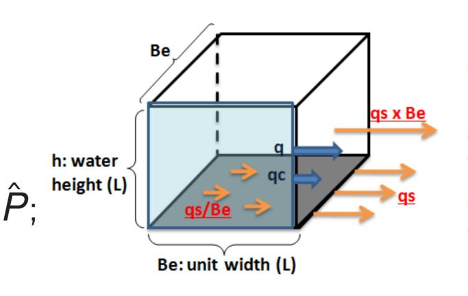
q: unit flow rate of water = va \* h (L<sup>2</sup>/T); c: critical unit flow rate of water (L<sup>2</sup>/T); qs: total sediment transport
