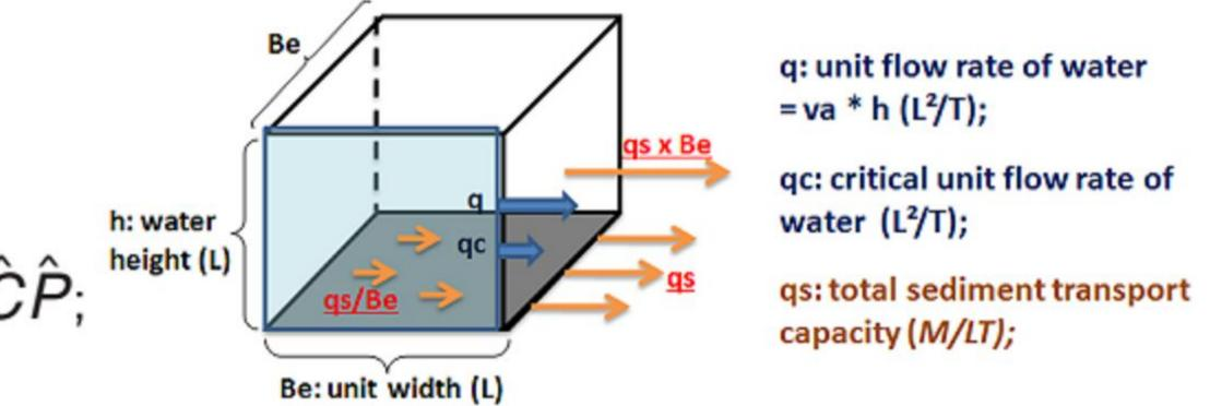
FIG 2, Conceptual view of "transport capacity".
