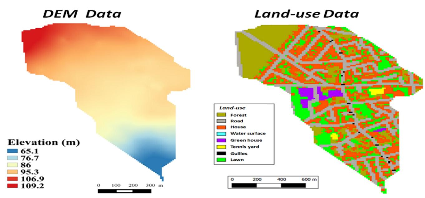
The surface area of this catchment is 0.72 km<sup>2</sup>,8 different types of land-uses, input grids resolution is 10m. The separate sewer system of the catchment is described in the FIG.3 (black line of the low-right graph).
