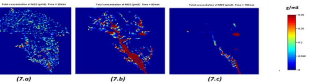
FIG 7, Total Suspended Solid concentrations on the surface grids; 7.a, time = 30 min, 7.b, time = 60 min, 7.c, time = 90 min,
