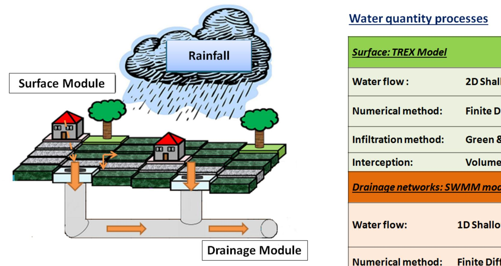
FIG 1, The concept of the Multi-Hydro Platform.
