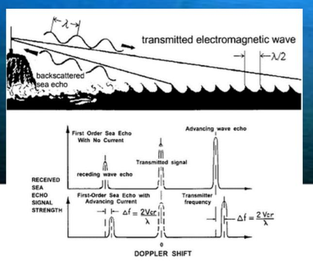
Bragg scattering from the sea wave whose wavelength one half of the radar wavelength, results in two discrete first order Doppler peaks in the sea-echo
