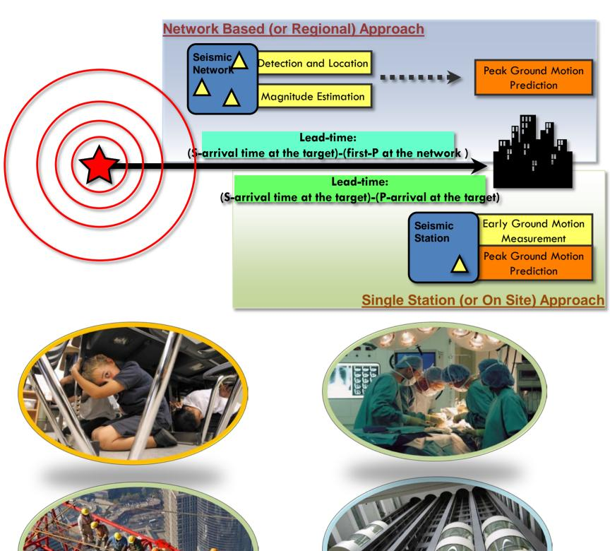
Earthquake early warning systems (EEWS) are Realtime, modern information systems that are able to provide rapid notification of the potential damaging effects of an ongoing earthquake, through the fast telemetry and processing of data from dense instrument arrays deployed in the source region of the event of concern (regional EEWS) or surrounding the target infrastructure (site-specific EEWS).
