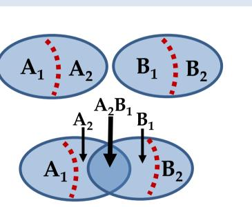
Optimal integration consists in increasing the *statistical efficiency* (subsets A<sub>1</sub>, B<sub>1</sub>) of the system's components (sets A, B) by: (a) minimizing the supply uncertainty of connected intermittent sources (i.e. wind) and **(b)** minimizing **excessive** output, via storage to a hub resource (water in the reservoir).
