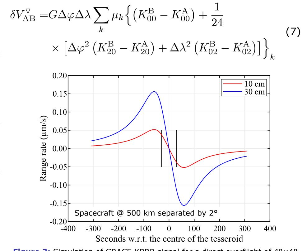
3: Simulation of GRACE KBRR signal for a direct overflight of 4°×4° urplus considering tesseroids of 10 and 30 cm of water column. The period of GRACE satellites is approximately 90 minutes and  $\pm 10^{\circ}$ corresponds to approximately  $\pm 154$  seconds (~0.067°/sec of latitude rate)
