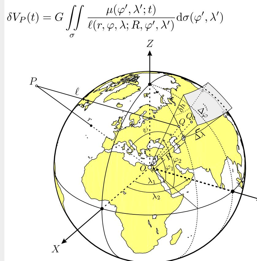
Figure 2: Geometry of a spherical tesseroid.
