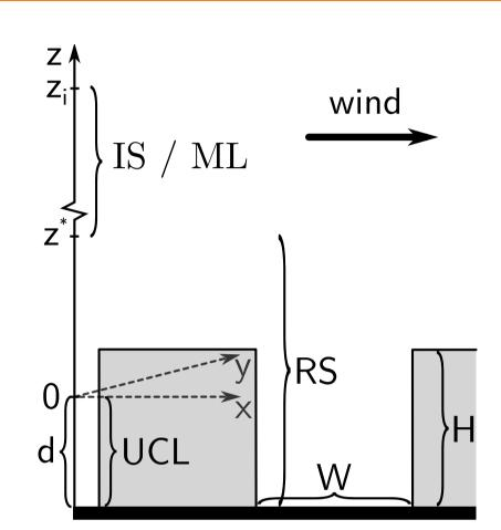
Model domain, coordinate system with zero plane displacement **d**, building height **H** and width **W**
