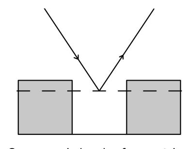
Conceptual sketch of a particle trajectory reflected at the zero plane displacement
