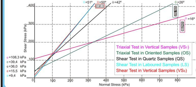
FG shows very low resistance to simple compression. Uniaxial tests show values of  $\sigma_c$  from 0,7 to 1,5 MPa. It was also obtained indirectly by triaxial tests. By this method  $\sigma_c$  fluctuates depending on the tectonic fabric orientation regarding to the axial stress ( $\sigma_c = 0,1 - 0,3 \text{ MPa}$ ).
