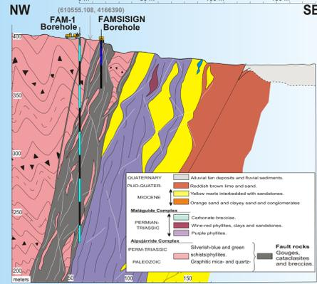
FAM-1 is a 175 m deep survey using wire-line continuous sampling (PQ-3, 83 mm) until 119,55 m, where the core diameter becomes HQ-3 (61 mm).
