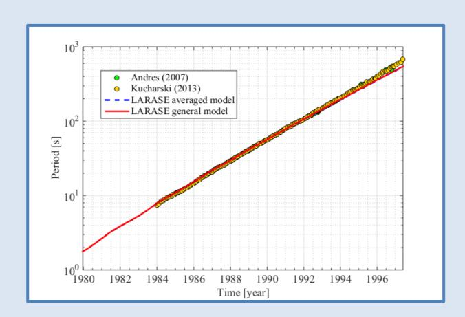
In the above figures we report for the older LAGEOS satellite the orientation (Right Ascension and Declination) and the rotational period that we have obtained applying our model LASSOS. The model is compared with two different sets of experimental data.
