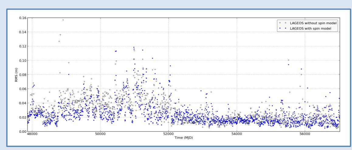
In this figure we have plotted for LAGEOS the root mean square (RMS) of the range residuals of a POD when the thermal forces are modeled (blue) with the use of LASSOS for the spin evolution, and when they are not modeled (black). The RMS reduces in average from 2.8 cm to 2.5 cm.
