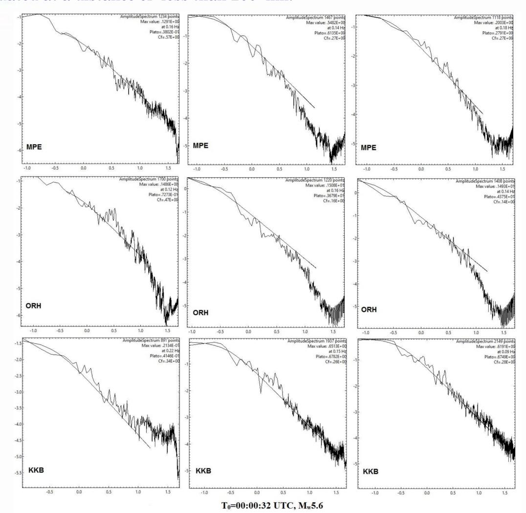
The results (based on P - wave and S - wave spectra) show that the stress drop mean value is about 53 bars for the P-wave and approximately 280 bars for the S - wave. The stress drop values estimated for P - waves are within the expected range for moderate earthquake while for the S - waves are several times higher than the expected ones.
