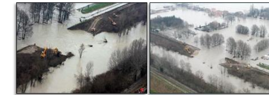
Fig. 2. Pictures of the breaching point on the right embankment of the Secchia river
