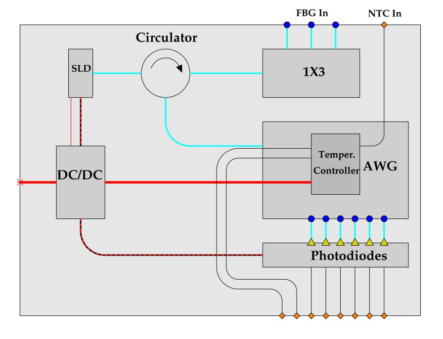
The data acquisition system is based on an electro-optic system that converts the FBG optical variations into voltage signals and a dedicated acquisition system: Geophysical Instruments for Low power Data Acquisition (GILDA)[3]
