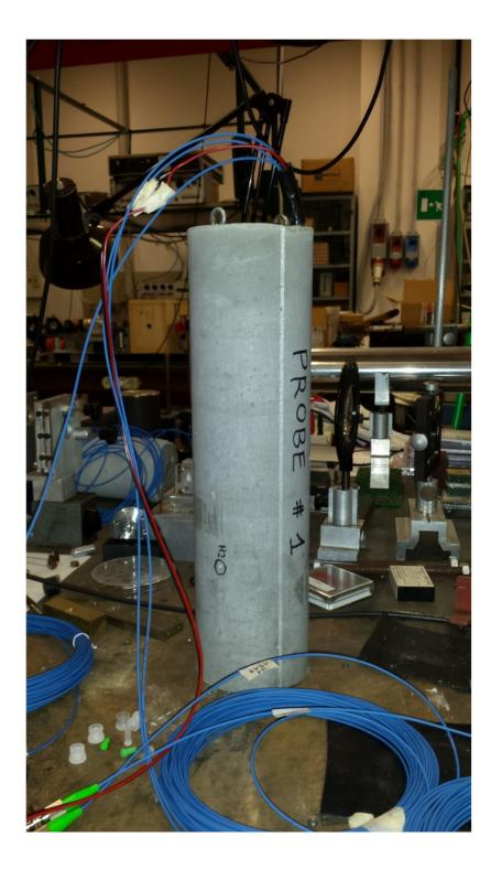
The final sensor set up consists in a concrete cylinder containing the three FBG and a NTC probe. The three fiber containing the FBG are encapsulated in three metallic tube, in order to maximize the sensitivity to the longitudinal stress and to protect the gratings. These three tubes are walled up in the concrete cylinder with the temperature probe.
