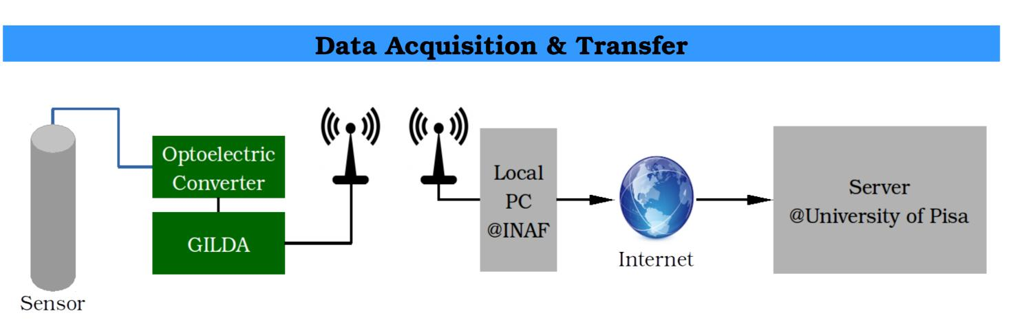
The optoelectronic converter is realized in order to exploit the S-Ratio algorithm[4] that allows to evaluate the bragg wavelength variation with a resolution higher than 0.5 pm (1 pm  $\approx$ ). The GILDA converts the electric signals into binary files every half an hour. These files are temporary stored in a pc located inside the INAF building. From here the data are sent to the University of Pisa server. Here we process and store the data in real time.
