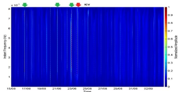
**Figure. 13:** The spectrum of the signals received from Tavolara, Italy (ICV) - 15-08-2016 to 02-09-2016. Green arrow denotes the disturbances - Red arrow denotes the occurrence of the earthquakes
