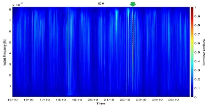
**Figure 14:** The spectrum of the signals received from Tavolara, Italy (ICV) - 15-10-2016 to 25-10-2016. Green arrow denotes the disturbances
