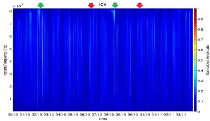
**Figure15:** The spectrum of the signals received from Tavolara, Italy (ICV) - 20-10-2016 to 03-11-2016. Green arrow denotes the disturbances - Red arrow denotes the occurrence of the earthquakes
