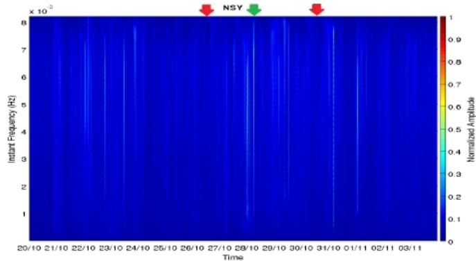
**Figure 19:** The spectrum of the signals received from Niscemi, Italy (NSY) - 20-10-2016 to 03-11-2016. Green arrow denotes the disturbances - Red arrow denotes the occurrence of the earthquakes
