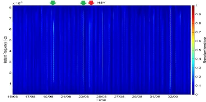
**Figure 17:** The spectrum of the signals received from Niscemi, Italy (NSY) - 15-08-2016 to 02-09-2016. Green arrow denotes the disturbances - Red arrow denotes the occurrence of the earthquakes
