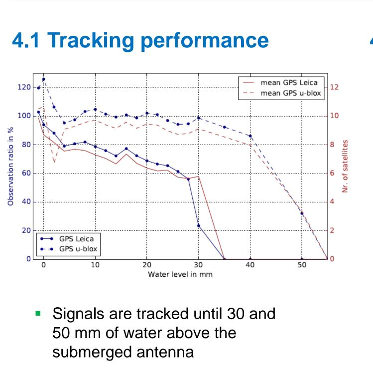
Low-cost receiver tracks generally more and longer than the submerged geodetic system
