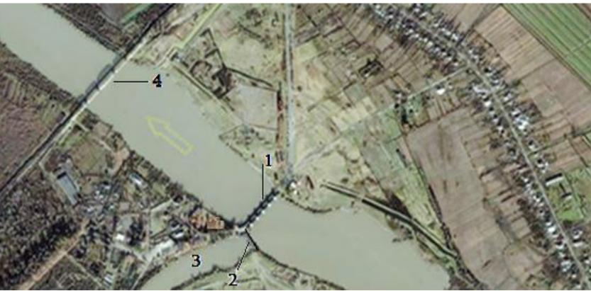
Fig.3. The water dividing dam on the river Rioni. 1. Dam; 2. Gateway regulating the water supply from the river Rioni to the City Channel. 3. City channel; 4. Railway bridge. The pointer indicates the main flow in the direction of the sea.
