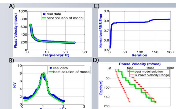
Figure 5. A) Dispersion curve B) Ellipticity curve C) Changing of NRMS error with iteration D) Estimated phase velocity-depth model.
