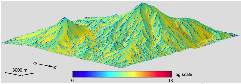
Catchment area is an area CA of a closed figure formed by a contour segment b at a given point of the topographic surface and two flow lines  $l_1$  and  $l_2$  coming from upslope to the contour segment ends.
