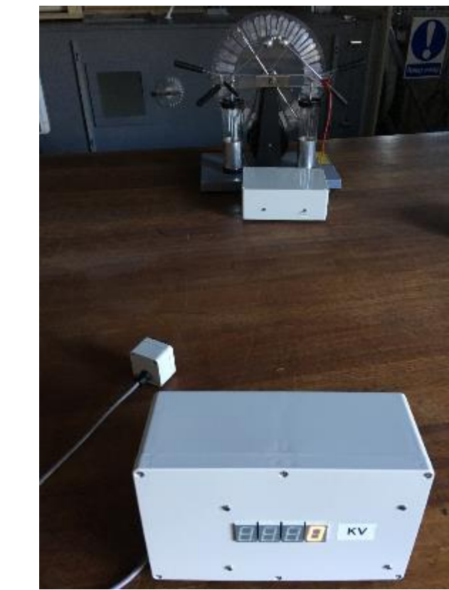
Fig 2 (left) A Wimshurst machine. Disks with multiple coupon electrodes counter-rotate, and generate a substantial charge by friction (middle) View of the electrodes, the spacing between which can be varied to find the breakdown distance at different potential differences (right) For safety, the potential difference across the electrodes is measured with an optically isolated voltmeter. The measurements are sent optically to a readout, on the student side of the bench.
