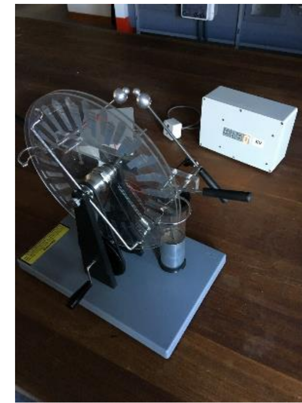
Fig 2 (left) A Wimshurst machine. Disks with multiple coupon electrodes counter-rotate, and generate a substantial charge by friction (middle) View of the electrodes, the spacing between which can be varied to find the breakdown distance at different potential differences (right) For safety, the potential difference across the electrodes is measured with an optically isolated voltmeter. The measurements are sent optically to a readout, on the student side of the bench.
