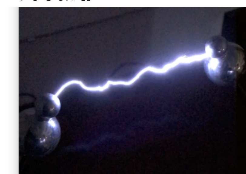
Fig 1 Typical discharge from the Wimshurst machine across a spark gap of 10 cm.
