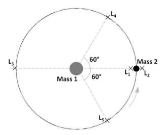
We use spacecraft located at the Sun-Earth Lagrange points, as a physical reference frame and plan to perform time of flight measurements of electromagnetic signals traveling on closed paths between the points. This allows to
