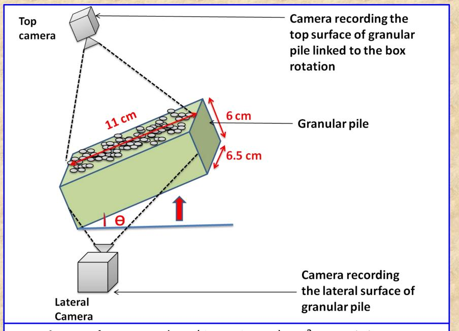
**Experimental setup**: A box (6.5 x 6 x 11) cm<sup>3</sup> containing monodisperse polystyrene or glass beads is slowly tilting by a motor to get the first and the successive avalanches. A lateral camera images the lateral surface of the granular pile. And a top camera images the top surface of the granular pile. The higher wet environment is created by saline solutions on which granular piles are placed for a week.
