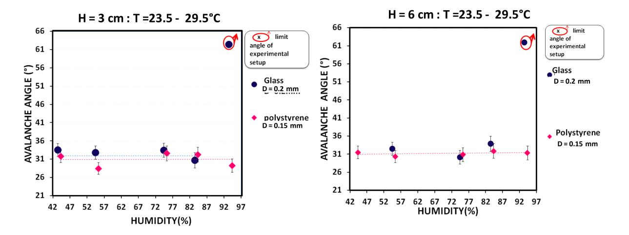
• Moisture acts strongly on the avalanche angle  $\Theta_M$  of glass beads D = 0.2 mm. and weakly on the  $\Theta_M$  of glass beads D = 0.5 mm  $\rightarrow$  The evolution of the angle as a function of humidity has the same trend as in [2];
