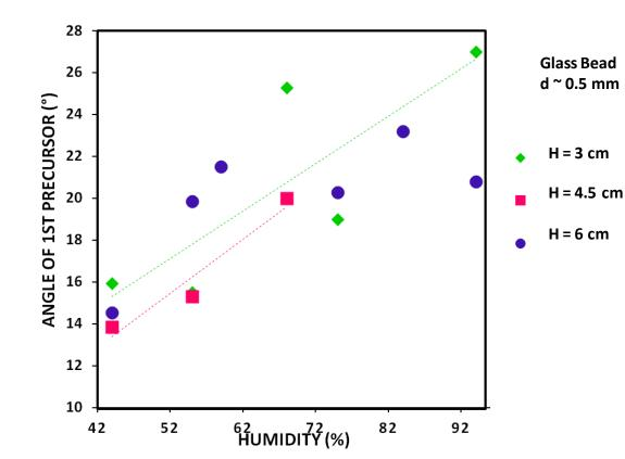
><u>Hypothesis</u> explaining the difference between our results and the results of [2] (who get  $\Theta_M$  (94%) = 85°) for grains with diameters D = 0.5 mm and H = 6 cm:  $\rightarrow$  Different sample preparation times between our experiment (1 week in a humid environment) and the experiment of Gomez (2 weeks)
