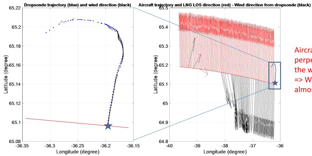
Aircraft was flying perpendicular to the wind direction => Wind and LOS almost collinear
