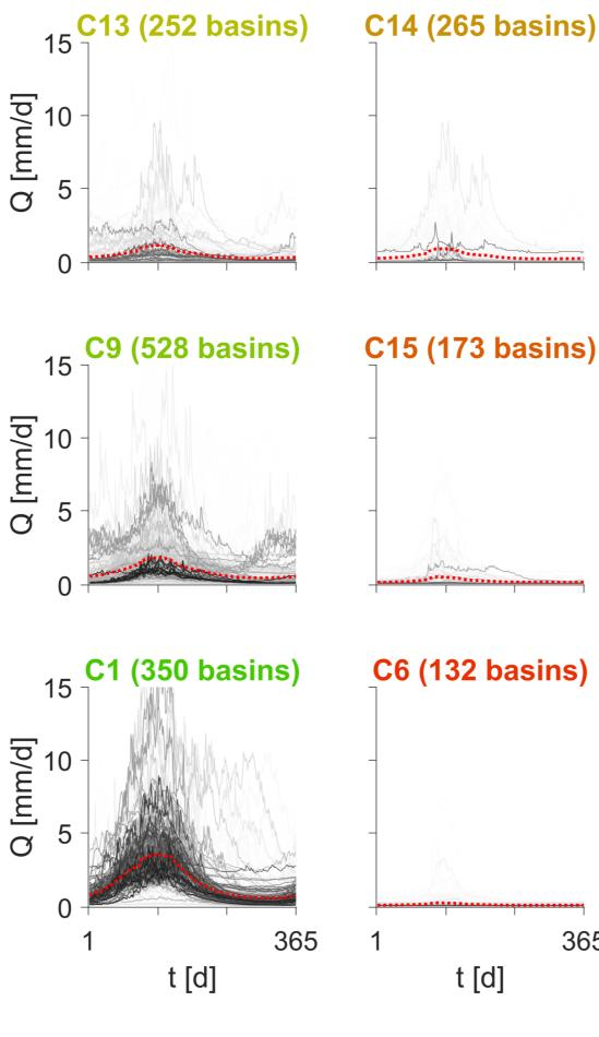
(fig. 4): flows grouped and shaded by climatic similarity between each basin and each reference climate. Per reference climate, only flows with similarity > 0.1 are shown, along with the similarity-weighted mean (...). Columns show how various gradients in climate space affect seasonal flow regimes in basins associated with these climates.
