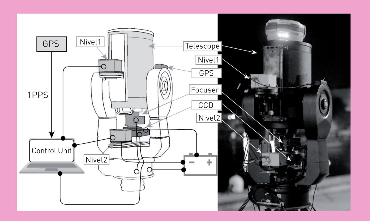
The preliminary astrogeodetic test observations were conducted by The ACSYS v2 in the main station (ITU test point) for 5 nights.
