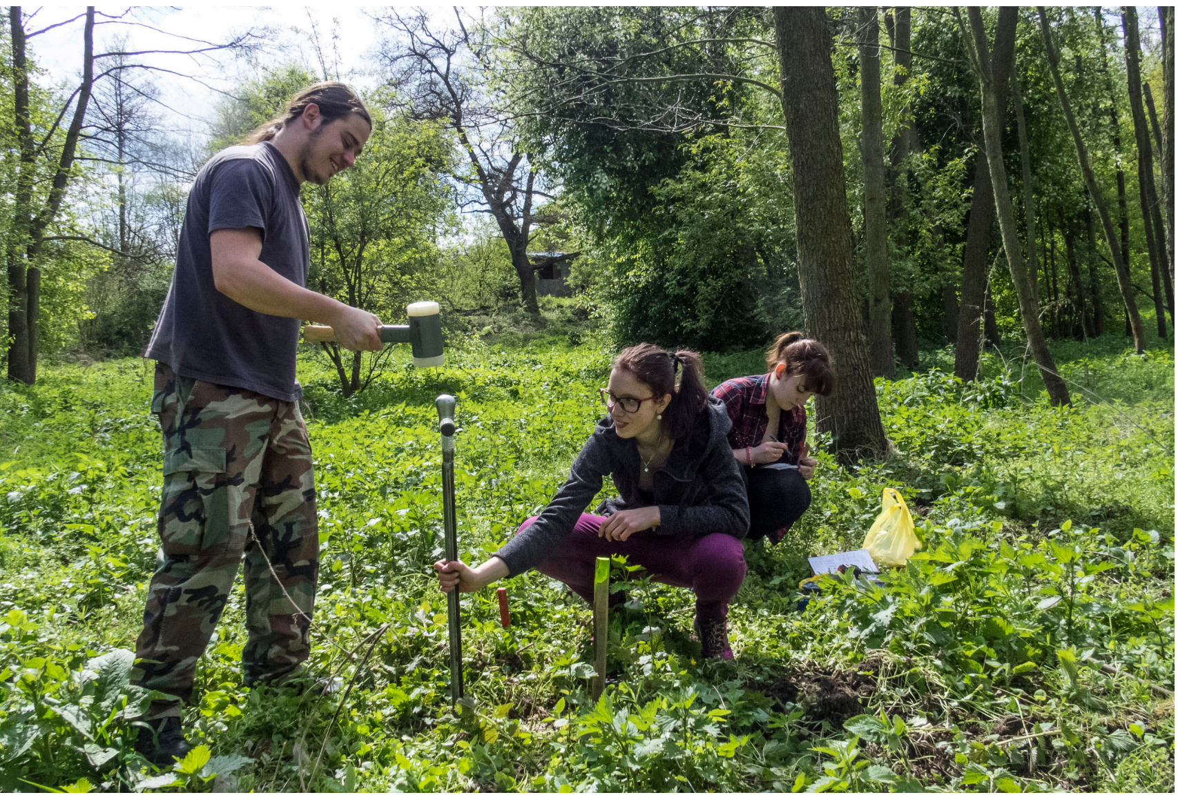
Fig. 7: Students sampling with core sampler.
