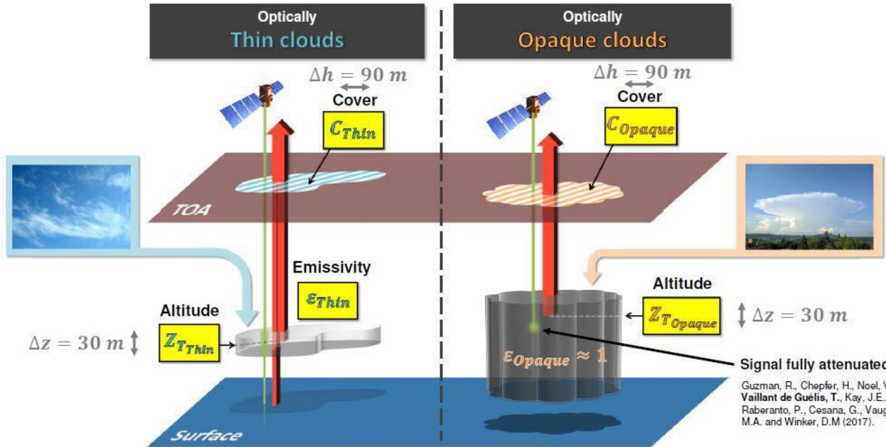
5 fundamental cloud properties observed by space-lidar to build a simple expression of the LW cloud radiative effect
