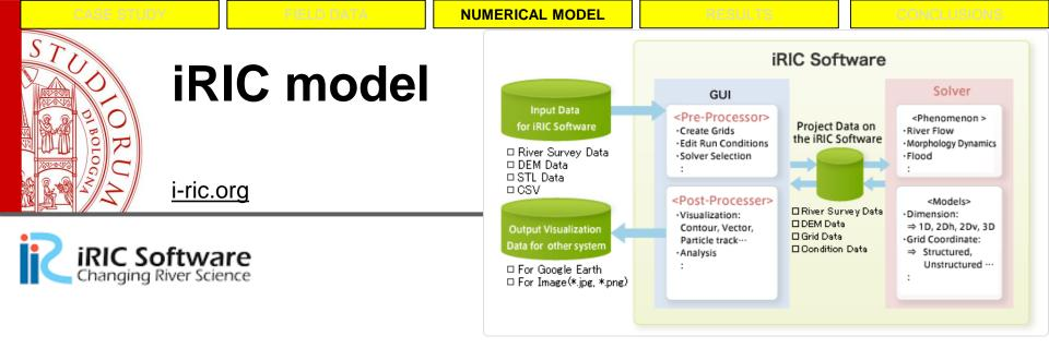
**iRIC** (International River Interface Cooperative) is a river flow and riverbed variation analysis software package combining the functionality of MD\_SWMS, developed by the USGS (U.S. Geological Survey) and RIC-Nays, developed by the Foundation of Hokkaido River Disaster Prevention Research Center.
