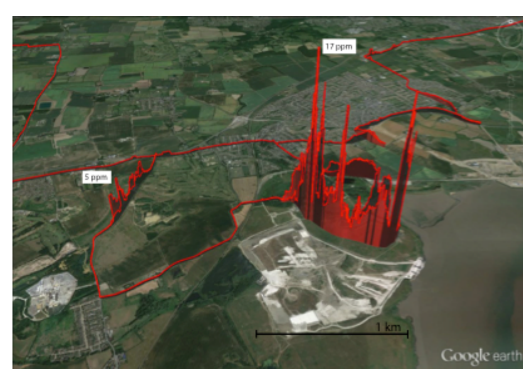
Detection of CH 4 plumes during mobile CH 4 measurements around the Mucking landfill site near London, UK (Zazzeri et al. 2015)
