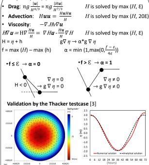
Computed mesh with 2412 Evolution of the free triangles, size of 10 - 100 km,  $\eta_o = 2$  m & h = 50 m Center with  $\mathcal{E} = 0.01$  m The free surface evolution by the numerical model is
