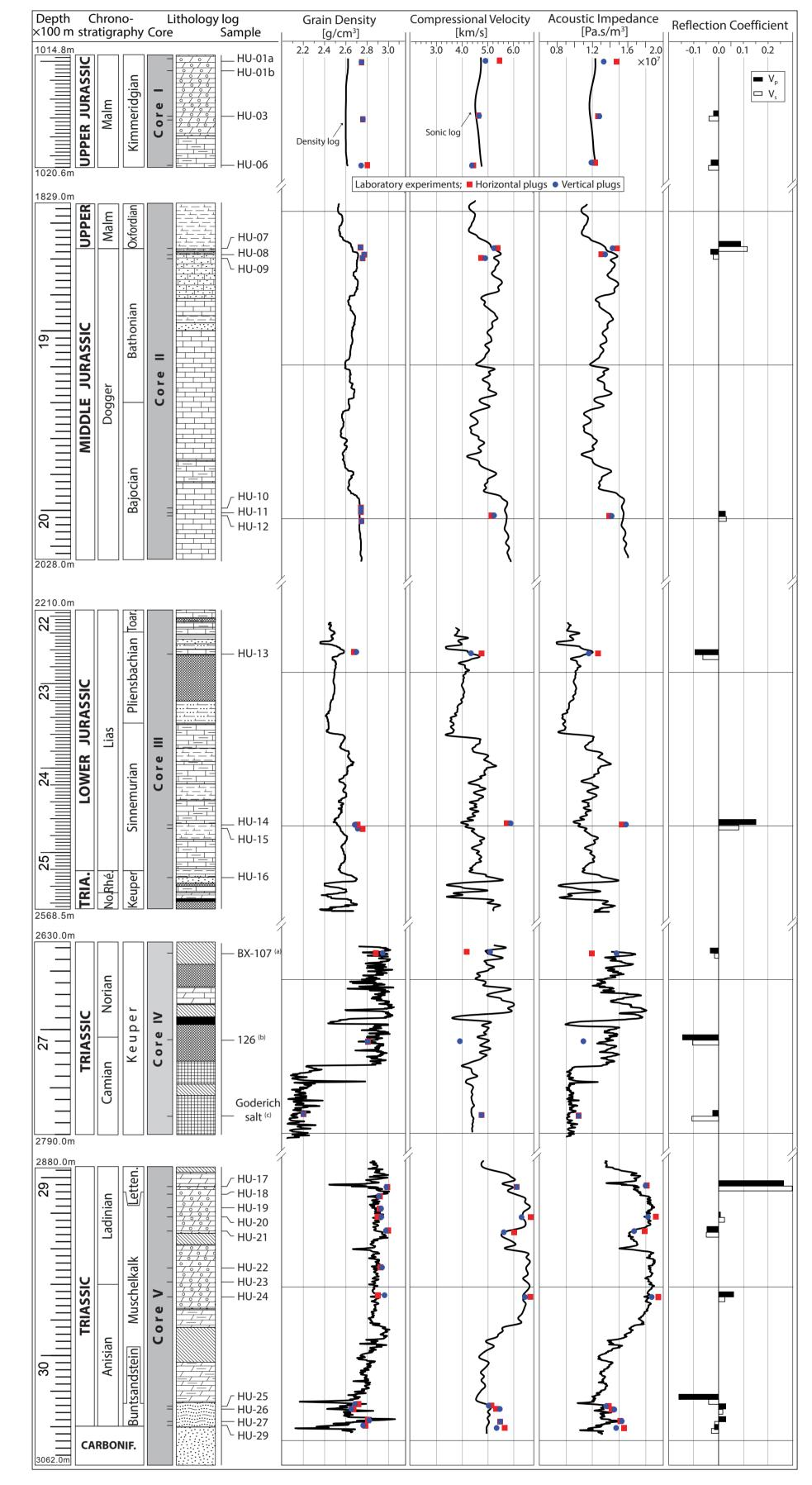
Fig D.5: Intregration between laboratory measurment and well-loggings.
