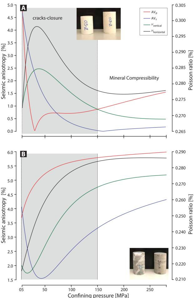
Fig D.2: Two examples (A: sample HU03, B: sample HU20) of dynamic seismic anisotropy and Poisson ratio corresponding to confining pressure.
