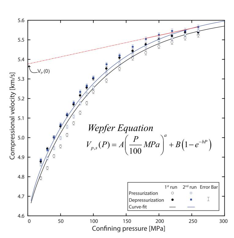
Fig D.1: Example of velocity measurments under two successive cycle of pressurization-depressurization Sample HU25X; depth 3028.3 m.
