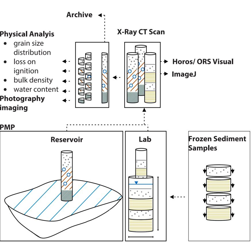
**Figure 2.** Schematic representation of core processing of lab and field cores.
