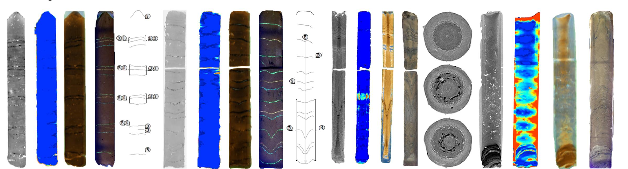
Figure 8. Coring Disturbances of lab Core #1, #2, Urft Core #1 and Urft #3. Core visualization (from left to right): CT image, Zeff, 3D-visualization, core image and digitized sediment layer (B = bending, S = smearing and E = expansion).
