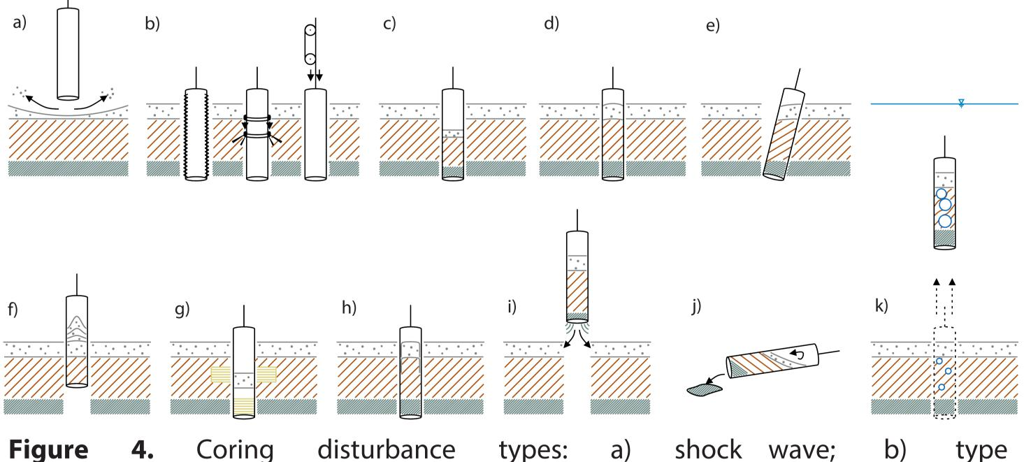
disturbance types: of penetration (vibra coring, hammering, pulley system); c) shortening; d) bending; e) tilting; f) expansion; g) entry deficit; h) smeaing; i) retrieval; j) handling and k) depressureization.
