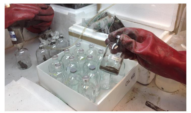
Figure 5. Laboratory sediment incubation.
