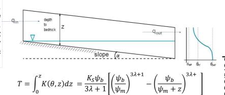
Soil Water Content in the soil profile was computed using a balance equation, while the SWC up to a specific depth z' (to allow comparisons with the measurements) was calculated using an analytical integral.
