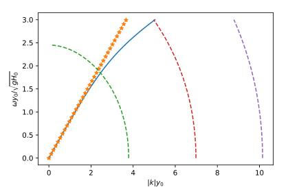
Fig. 1: The dispersion relation in infinite channel with parabolic cross-section. Broken curves means that wave vector is purely imaginary (associated modes grow exponentially in +x direction). The stars are the dispersion relation given by  $\omega = \sqrt{g^2 H_0/3} k$  where  $2H_0/3$  is the averaged depth of the parabolic channel.
