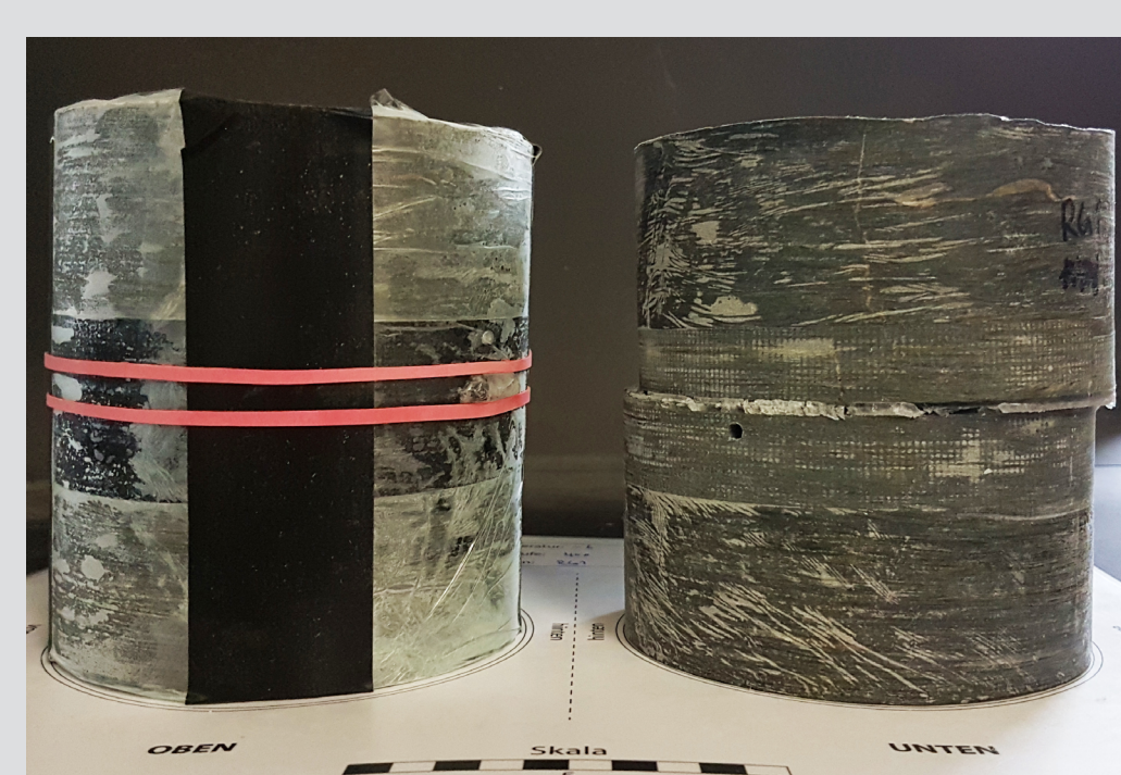
Prepared and sheared sandwich sample.
