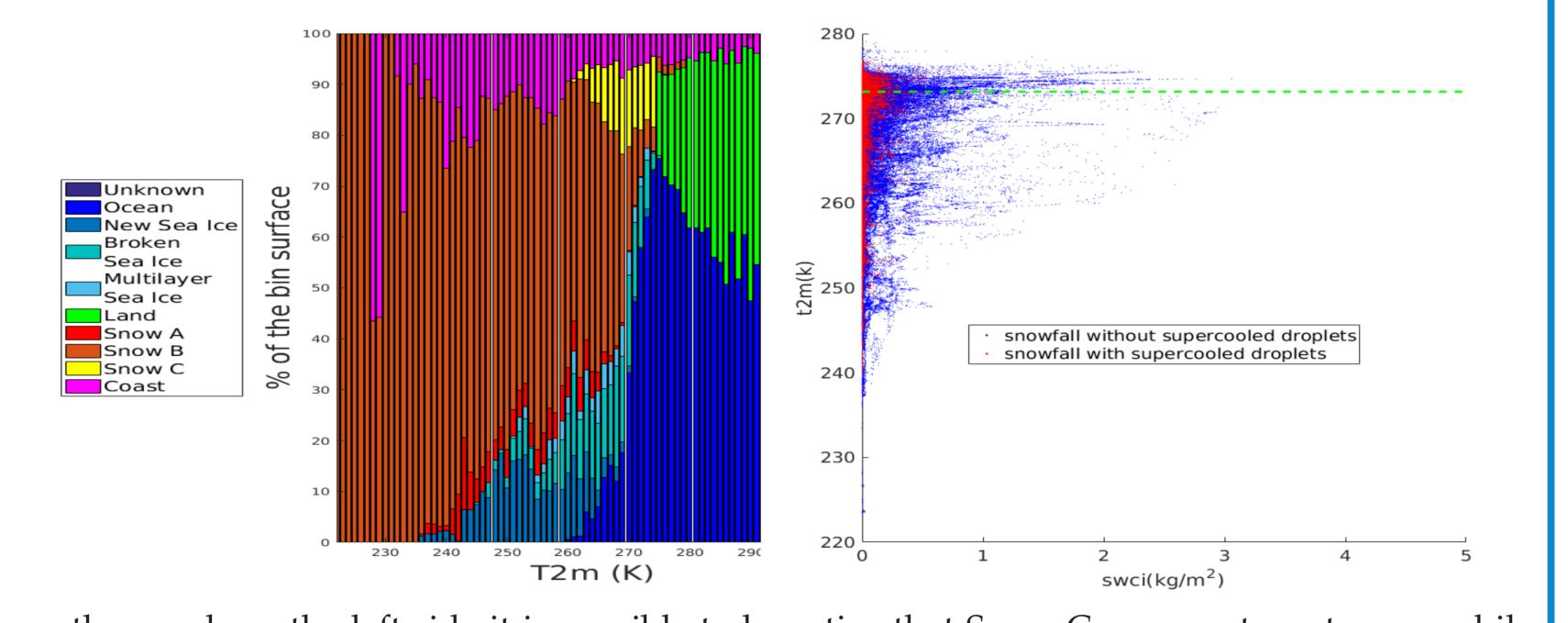
From the graph on the left side it is possible to hypotize that Snow C represents wet snow while snow A and snow B represent dry snow, because Snow C is linked to warmer situations. By the graph on the right side it is possible to observe that the presence of supercooled droplets on the cloud top layers characterizes light snowfall events.
