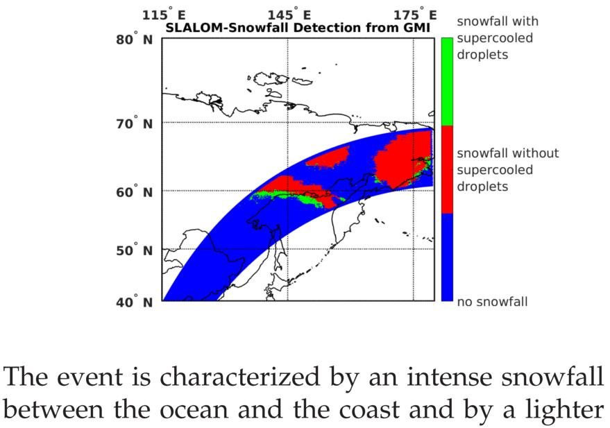
between the ocean and the coast and by a lighter snowfall event over the internal regions. Both DARDAR data and SLALOM detection product show the presence of supercooled droplets on the cloud top in the southern part of the event and the GMI surface classifier identifies a dry snow cover (snow B) on the continental part It is possible to observe that:
