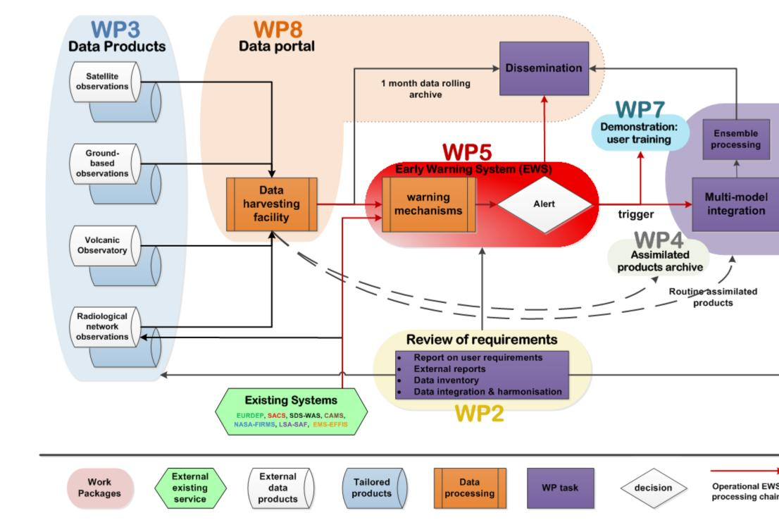
The data flow chart of EUNADICS-AV divided into the original project work packages. Data provided by the volcano observatories is processed by the data harvesting facility and is utilised both as an input and as a control.
