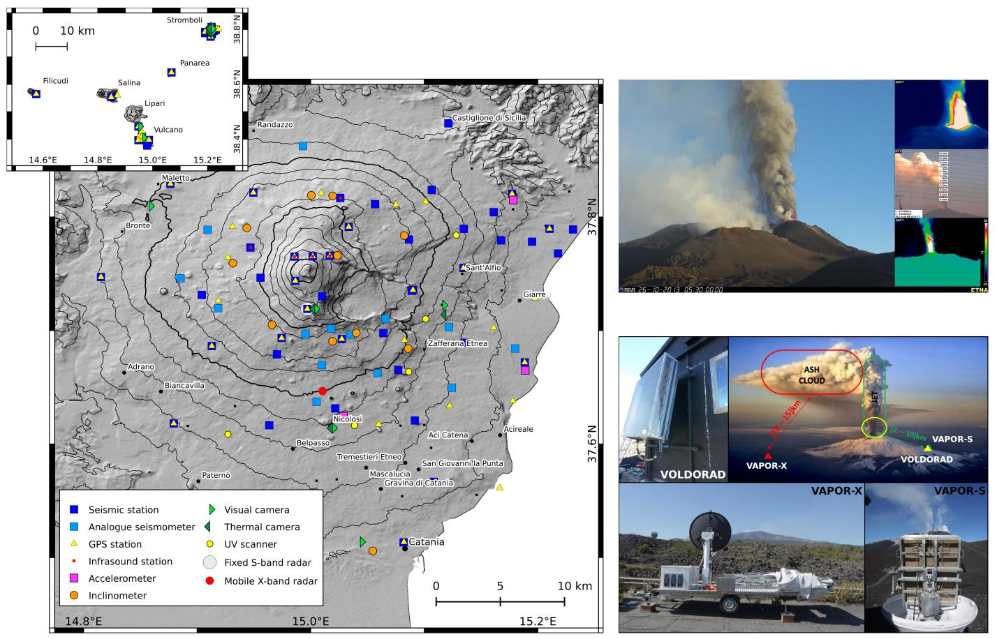
Plume features are measured through either calibrated visual/thermal cameras or by radar. The novel radar setup includes fixed S- and Lband instruments for measuring flux rates, and a mobile X-band instrument for analysing the downwind ash cloud.
