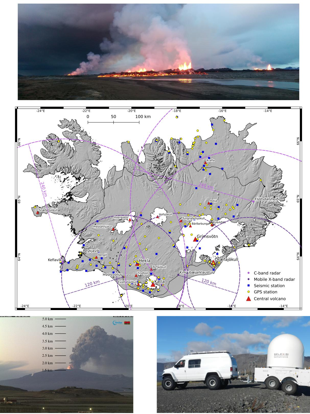
During the 2010 eruption of Eyjafjallajökull, calibrated web cameras were placed in order to measure the plume height<sup>[2]</sup>. Now a new automated plume height retrieval system, VESPA, uses data from Iceland's two fixed position C-band radars, and two mobile X-band radars (shown above). Future data products will include real-time ceilometer and lidar measurements.
