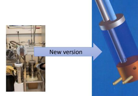
Twin traps, manual version being replaced by temperature controlled version
