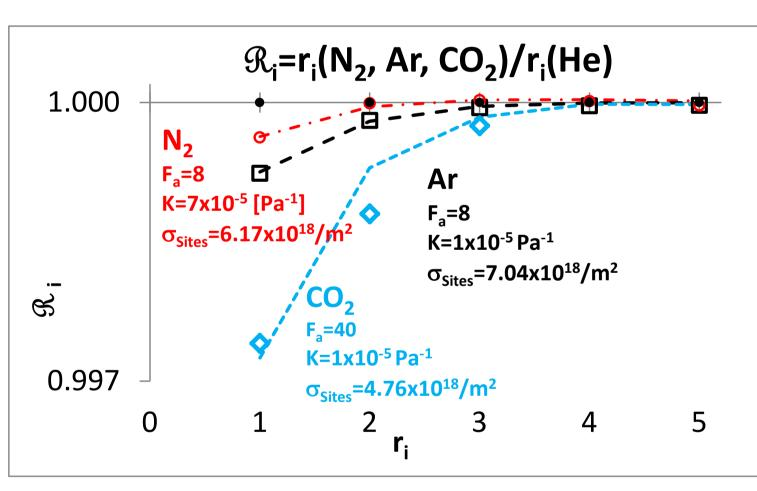
Fit of minor volume ratios measurements with several gases using a Langmuir model
