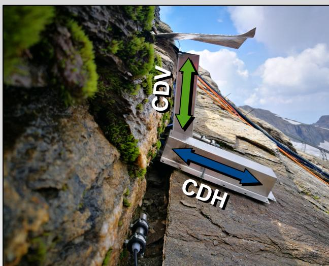
**Crackmeter measurements** Geokon Model 4420 Vibrating Wire Crackmeters measure horizontal (CD<sub>H</sub>) and vertical crack deformation (CD<sub>V</sub>) as well as crack top temperature (CTT).
