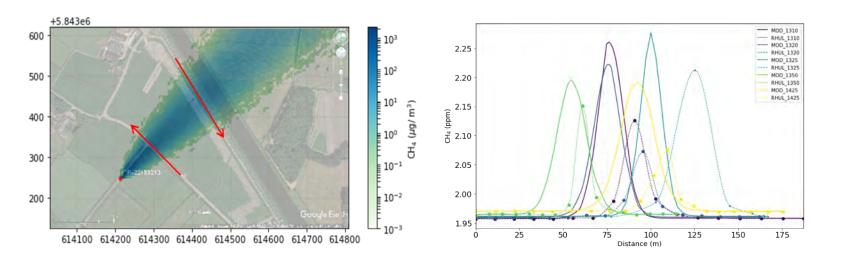
Left: GRAL simulated CH<sub>4</sub> concentration (5-minute average) during a tracer release experiment in February 2018. The red arrows denote the paths of the mobile measurement platforms crossing the plume multiple times at two distances from the source. Right: Simulated (solid lines) and measured (dotted lines with symbols) CH<sub>4</sub> mole fractions along different transects sampled by the car of RHUL. Matching the areas below the curves allows estimating the strength of the source.
