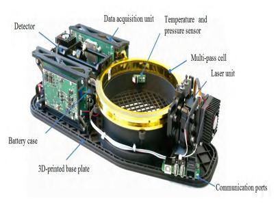
Sensor based on open-path direct absorption spectrometry, using a single-mode quantum cascade laser (DFB-QCL)
