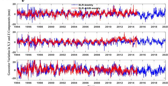
Figure 1 Time series of geocenter motion estimated by this study and AIUB
