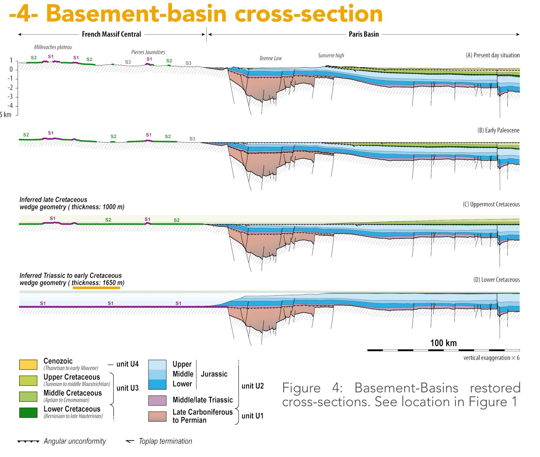
Coupling between AFTA thermal modelling and cross-section reconstruction, allows to estimate a geothermal gradient (i.e. between 30 to 45°C.km-<sup>1</sup>) and calculate denudation rates.
