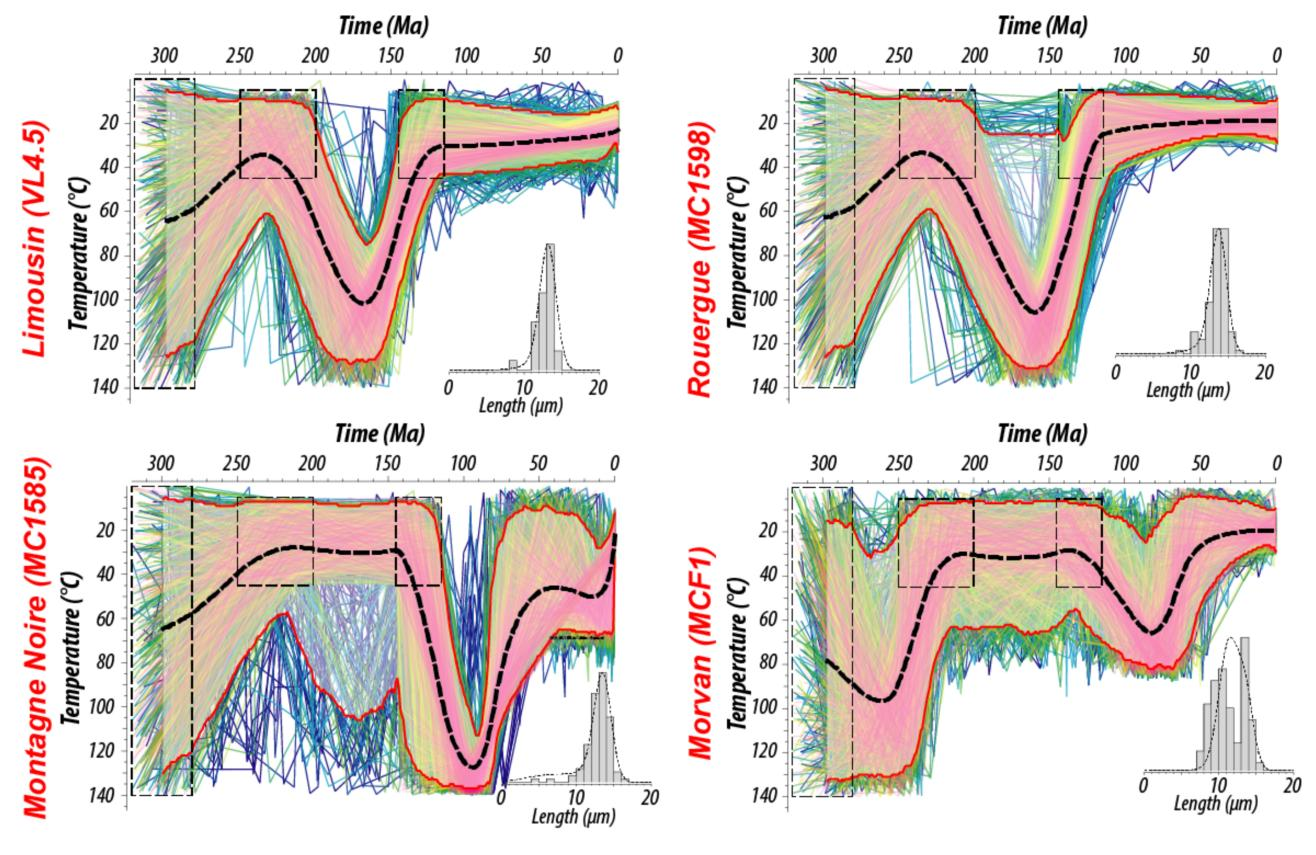
Figure 3: Results thermal modelling using QTQt (Gallagher 2012) carried out on the samples with more than 75 confined tracks measured. Modelling results are displayed in a timetemperature diagram and frequency distribution of measured confined track length. The dashed square represents the constraints applied to the modelling (i.e. planation surfaces). The bold dashed line is the best-fit cooling path.
