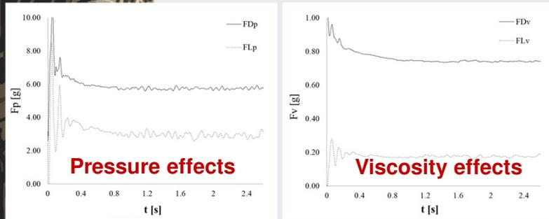
Figure 2. Integrated pressure and viscosity forces (grouped as drag and lift, in accordance to traditional convention) as a function of time, for Re=5000
