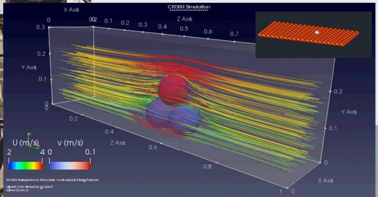
Figure 3. Coupled CFD-DEM simulation with moving particle; future set up with rough-bed conditions (inset)
