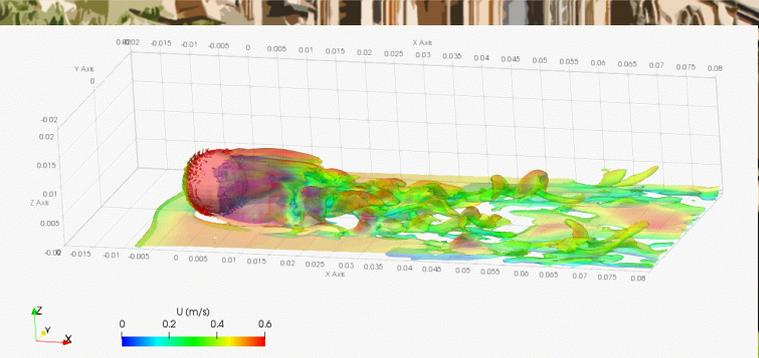
Figure 1. Vortex structures behind a sphere on a smooth bed; Re=5000; Q-criterion = 100
