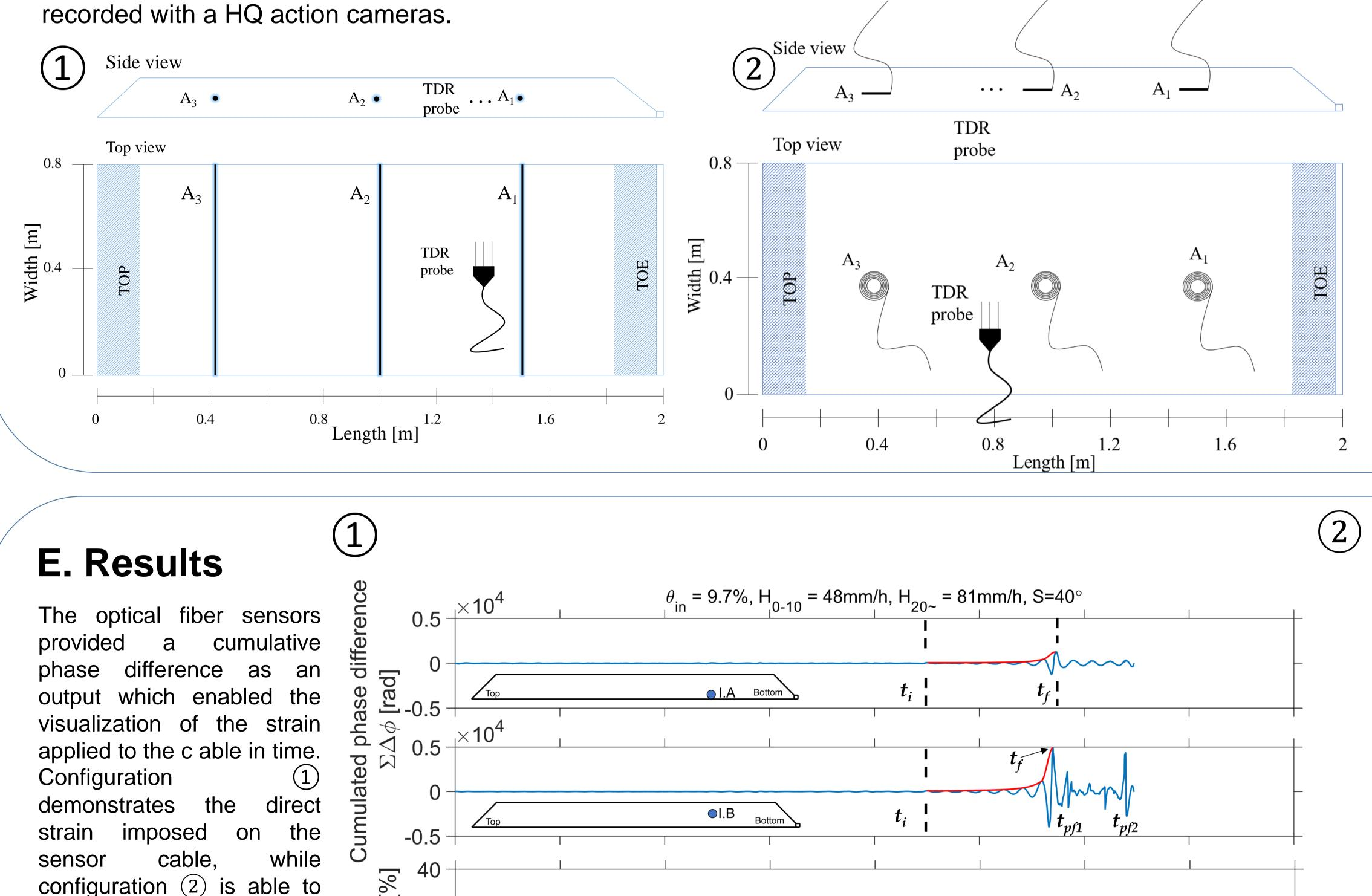
configuration (2) is able to detect high frequency response of the sensor due to the interparticle friction of grains. Spectral analysis illustrates this response.
