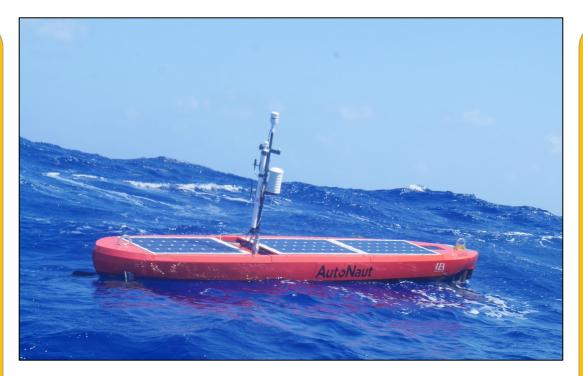
Powered by three 100 W rated solar panels charging four lithium ion batteries
