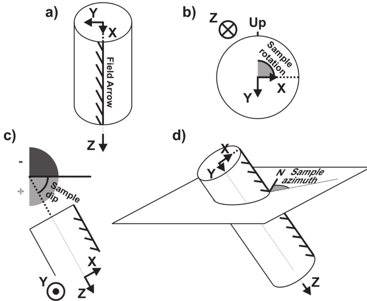
Figure 3: Sample coordinate system. (a) Relation of the sample coordinate system with the field arrow. (b) Measurement of the sample rotation angle. We also refer to X as the 12 o'clock position. (c) Measurement of the sample dip angle. (d) Measurement of the sample azimuth angle.
