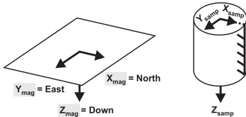
Figure 4: Correction parameters for different orientations of the sample ( $X_{\text{samp}}$ ,  $Y_{\text{samp}}$  and  $Z_{\text{samp}}$ ) in the magnetometer ( $X_{\text{mag}}$ ,  $Y_{\text{mag}}$  and  $Z_{\text{mag}}$ ), part 1 ( $Z_{\text{samp}} = \pm Z_{\text{mag}}$ ). The correction azimuth, dip and rotation are measured as if the X, Y and Z coordinates of the magnetometer were respectively attributed to the North, the East and the downward direction.
