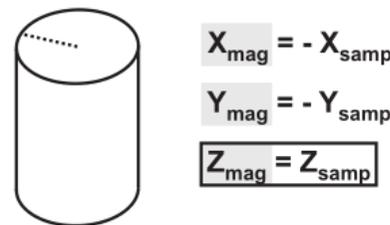
Correction azimuth = 180
