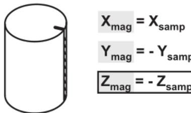
Correction azimuth = 180
