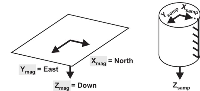
Figure 5: Correction parameters for different orientations of the sample ( $X_{\text{samp}}$ ,  $Y_{\text{samp}}$  and  $Z_{\text{samp}}$ ) in the magnetometer ( $X_{\text{mag}}$ ,  $Y_{\text{mag}}$  and  $Z_{\text{mag}}$ ), part 2 ( $Z_{\text{samp}} = \pm X_{\text{mag}}$ ). The correction azimuth, dip and rotation are measured as if the X, Y and Z coordinates of the magnetometer were respectively attributed to the North, the East and the downward direction.
