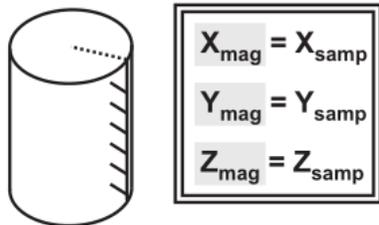
Correction azimuth = 0
