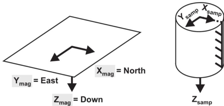
Figure 6: Correction parameters for different orientations of the sample ( $X_{samp}$ ,  $Y_{samp}$  and  $Z_{samp}$ ) in the magnetometer ( $X_{mag}$ ,  $Y_{mag}$  and  $Z_{mag}$ ), part 3 ( $Z_{samp} = \pm Y_{mag}$ ). The correction azimuth, dip and rotation are measured as if the X, Y and Z coordinates of the magnetometer were respectively attributed to the North, the East and the downward direction.
