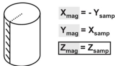
Correction azimuth = 90
